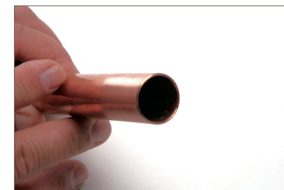
Figure 13.8. Reamed and deburred branch tube end
