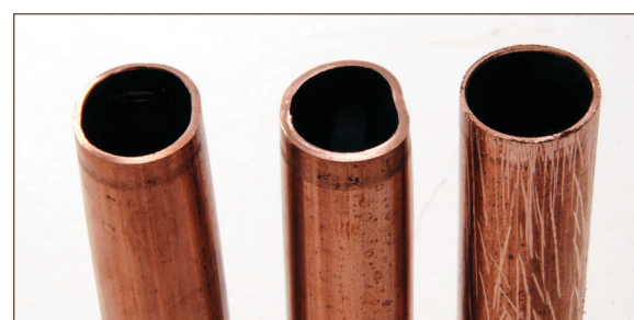
Figure 11.4. Inspect tube for imperfections
