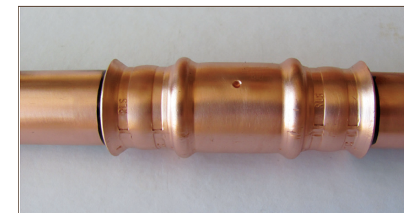
Figure 11.17. Completed joint showing double 360° crimps
