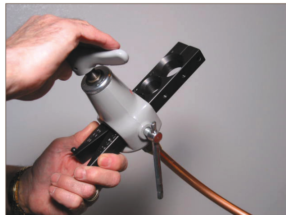
Figure 9.4. Lowering the Flaring Cone Into the Tube End
