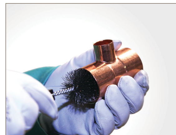
Figure 7.8. Cleaning: Fitting Brush
