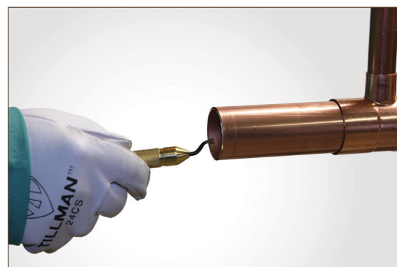
Figure 7.5. Reaming: Deburring Tool
