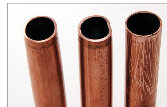
Figure 10.1. Inspect tube for imperfections
