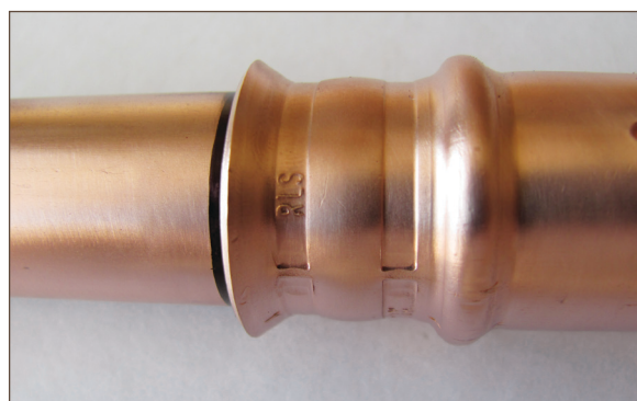
Figure 11.20. Press jaw crimp mark
