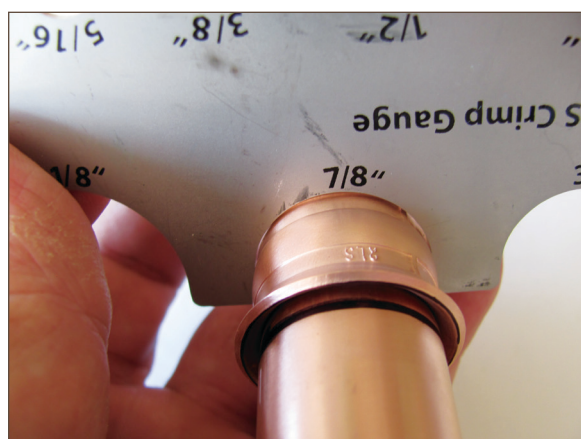
Figure 11.22. Correctly crimped fitting
