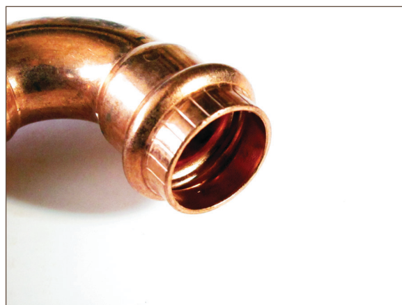
Figure 11.11. Press fitting (NOTE: Missing o-ring)
