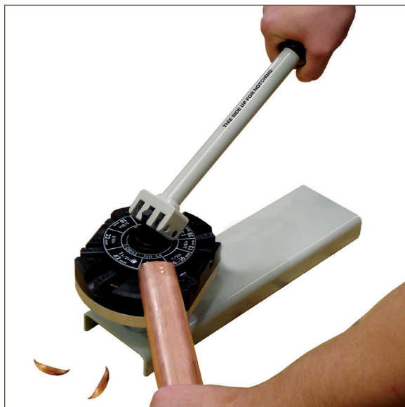
Figure 13.9. Using the notching and dimpling tool
