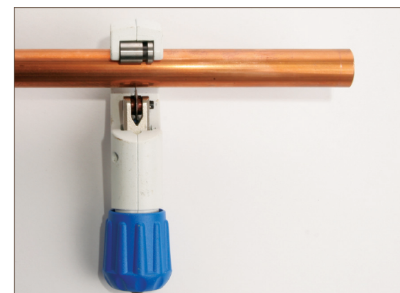
Figure 11.6. Cutting the tube square
