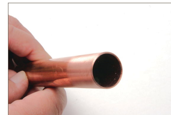
Figure 11.10. Properly prepare tube end
