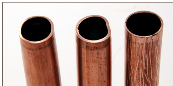
Figure 11.4. Inspect tube for imperfections
