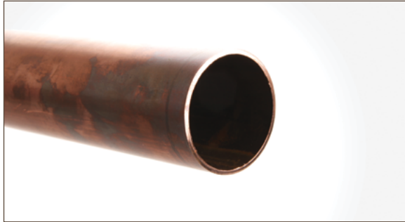
Figure 10.3. Square-cut tube end
