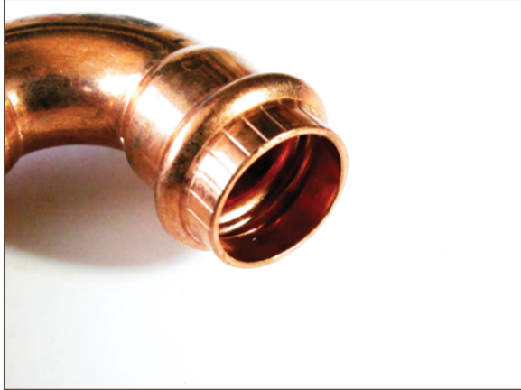
Figure 11.11. Press fitting (NOTE: Missing o-ring)
