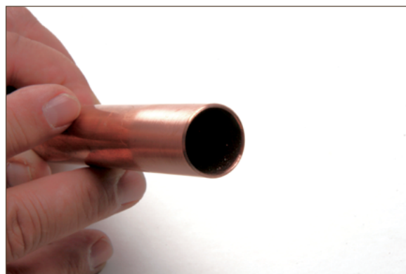
Figure 13.8. Reamed and deburred branch tube end
