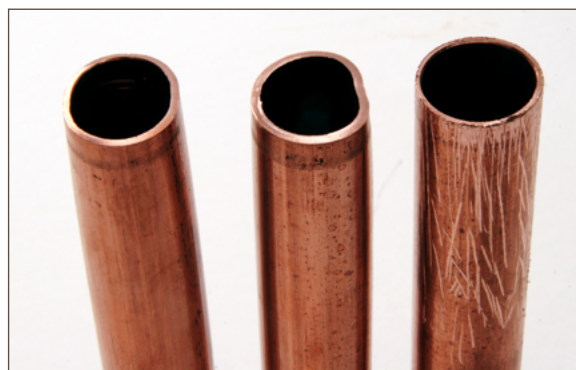
Figure 10.1. Inspect tube for imperfections
