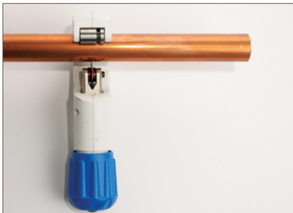
Figure 11.6. Cutting the tube square
