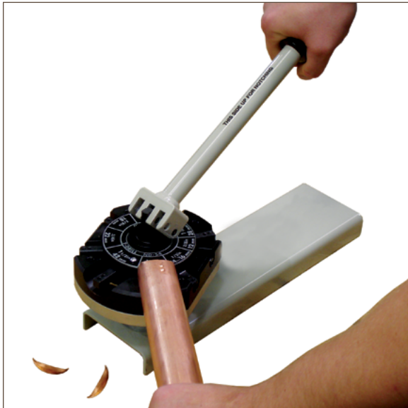
Figure 13.9. Using the notching and dimpling tool
