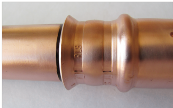
Figure 11.20. Press jaw crimp mark
