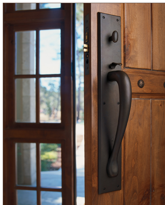
Figure 3.2B. The oxidized finish on this cast silicon bronze lockset produces a stable compound that inhibits corrosion and maintains its color.
