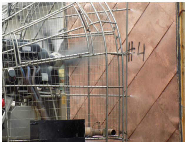
Figure 15.6.3: Diagonal copper flat lock cladding tested by the AAMA 501.1 dynamic pressure water penetration procedure.
