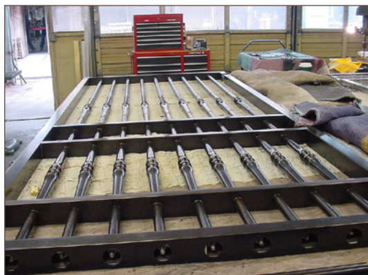
Figure 3.3B. Oil-rubbed bronze gates prepared for installation at the State Capital in Harrisburg, Pennsylvania.
