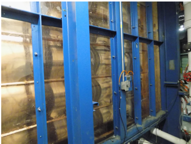
Figure 15.6.4: Horizontal single lock standing seam cladding tested for wind resistance according to the ASTM E330 test method.
