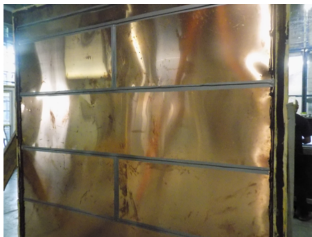
Figure 15.6.1: Horizontal copper flat lock panel with taped joints to isolate joinery elements for ASTM E283 air flow testing.
