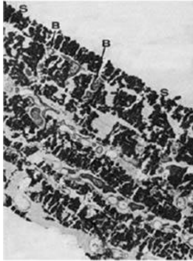
Figure 2: Transmission electron microscope micrograph of corrosion products of Cu-Ni exposed in Langstone Harbor after 22 weeks found B – bacteria between layers of corrosion products, S – no bacteria found on the surface (12,000:1)
